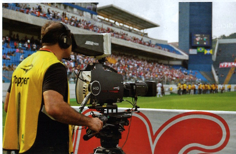
I-Movix's SprintCam Vvs HD now operates at frame rates up to 2,700fps in 1080i50 or up to 5,800fps in 720p60.
