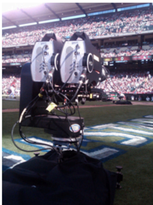
The slow-motion 3-D system uses twin SprintCam Vvs HD systems mounted on a PACE 3-D rig.
